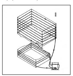
If part of the skin type condenser is used as an oil-cooling condenser, a tube layout like the one shown in fig. 11 may be used. If optimum oil cooling of the compressor is aimed at, approximately one half of the total tube length should be used as oil-cooling condenser.
