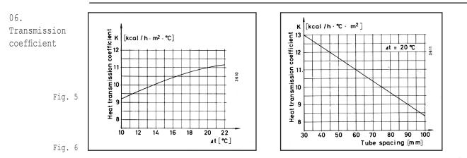
The transmission coefficient or U-value expresses the quantity of heat in kcal/h which can be removed per m at a temperature differential of  $1^{\circ}C$ .
