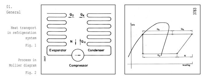
The object of the condenser in the refrigeration system is to remove the heat supplied to the refrigerant in the evaporator and during the compression in the compressor, as well as to condense the refrigerant vapours into liquid.
