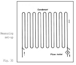
For a relative comparison between different compressor types or makes of condenser a setup like the one shown in fig. 30 can be used. Hater at a constant velocity and inlet temperature is fed through the condenser.
