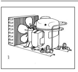
For domestic refrigeration appliances and small commercial refrigeration systems, the fan-cooled condenser is, normally, only used in connection with "fan-cooled condensing units" which consist of a condenser, a fan, and a compressor (see fig. 17). An example of this field of application is the chest freezer designed for tropical conditions where, with a statically cooled condenser, it can be difficult to provide space for the necessary condenser area.
