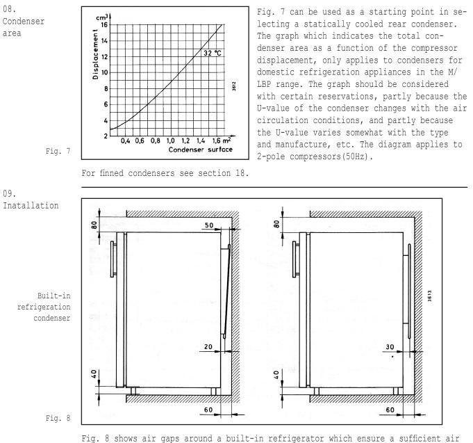
Fig. 8 shows air gaps around a built-in refrigerator which ensure a sufficient air supply to compressor and condenser. The distance to the rear wall of the refrigerator should be approx. 60 mm, and the condenser should be mounted in the centre of the air gap.
