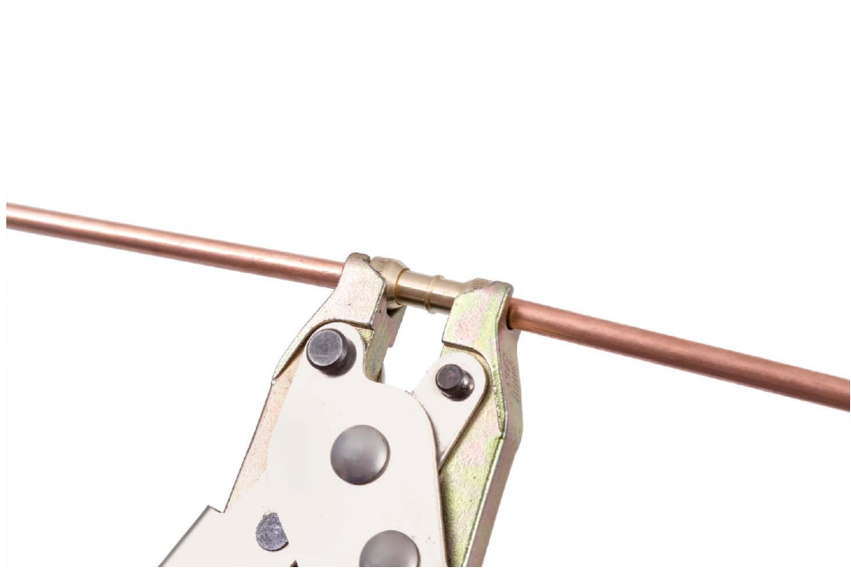
Image 4: With the pliers for manual assembly, a hermetic connection will be established due to pressure, source: VULKAN Lokring
