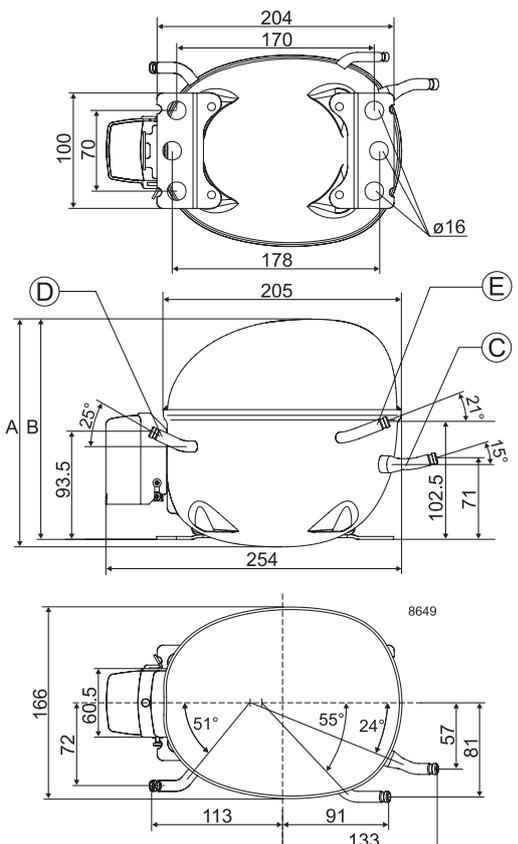
**EN 12900 Household (CECOMAF)** 220V, 50Hz, RC 3µF, 2W PTC consumption incl., static cooling
