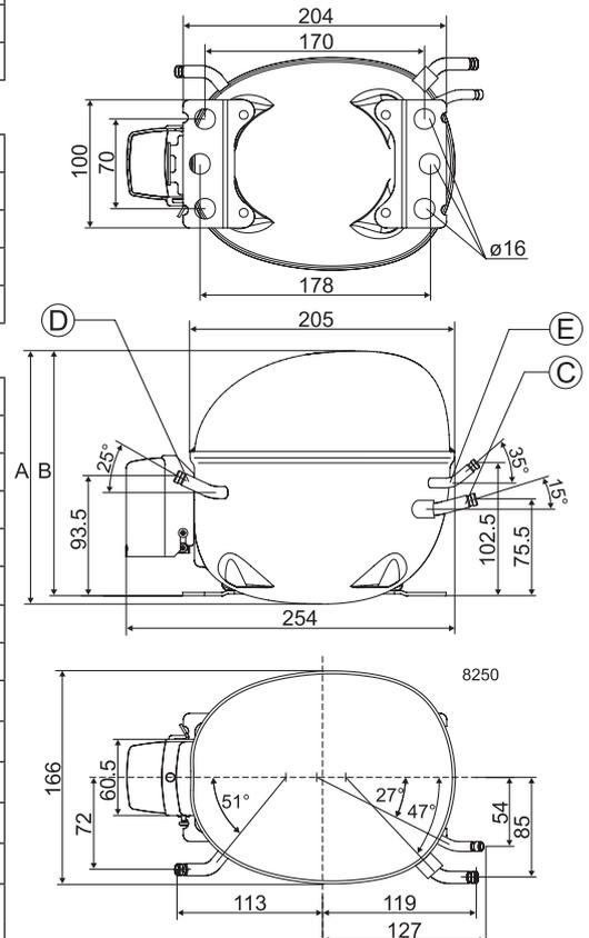
**EN 12900 Household (CECOMAF)** 220V, 50Hz, RC 4µF, 2W PTC consumption incl., static cooling
