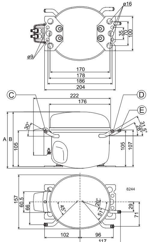
**EN 12900 Household (CECOMAF)** 220V, 50Hz, RC 4µF, ePTC consumption incl., static cooling
