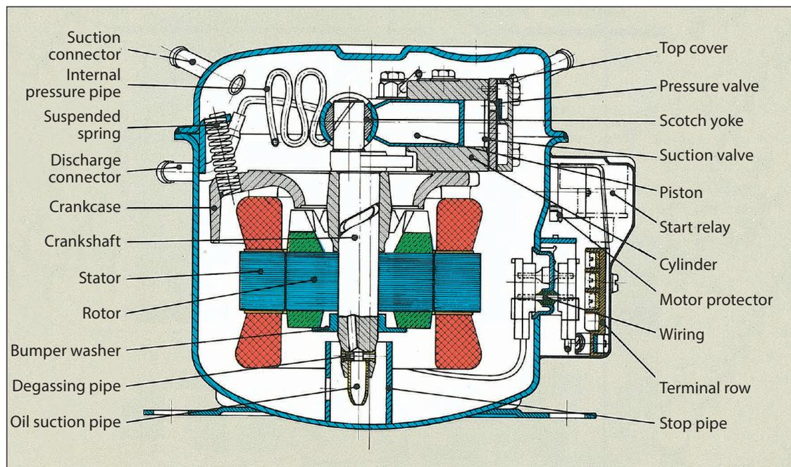
Cross-section of PW compressor.
