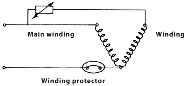
Wiring diagram with PTC and winding protector. ▲
