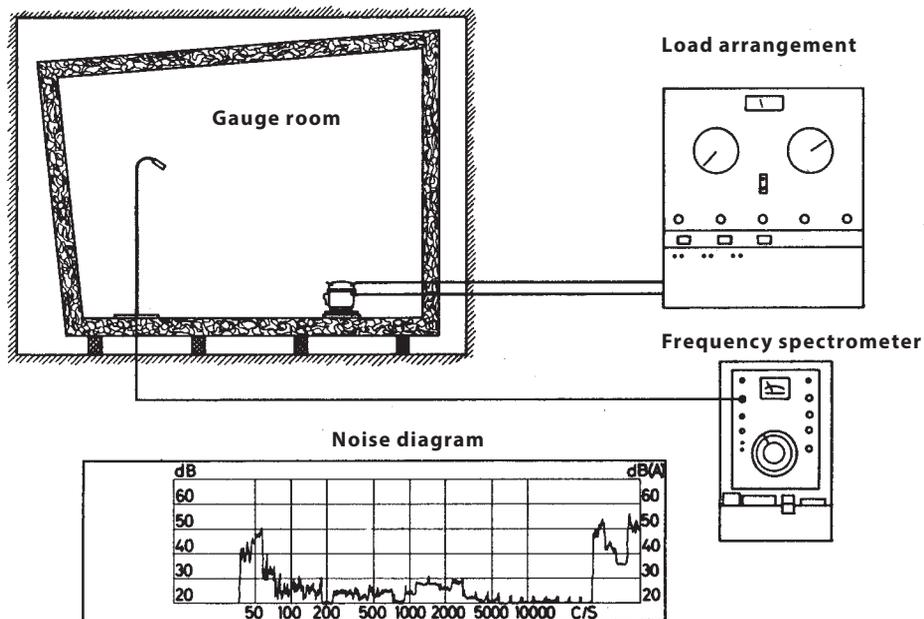
◀ Drawing of principle for noise measuring.
