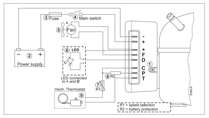
The electronic unit is a dual voltage device. This means that the same unit can be used in both 12V and 24V power supply systems. Maximum voltage is 17V for a 12V system and 31.5V for a 24V power supply system. Max. ambient temperature is 43°C. The electronic unit has a built-in thermal protection which is actuated and stops compressor operation if the electronic unit temperature gets too high.
