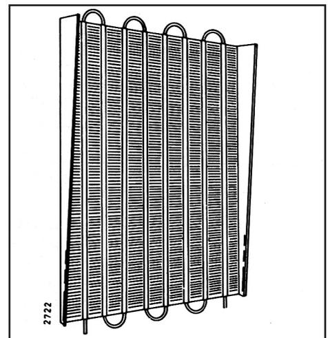
The rear condenser, which is primarily fitted on the back of the refrigeration appliance, is especially used for refrigerators and upright freezers, but in some cases also for small chest freezers.
