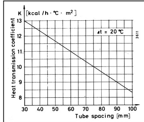
The transmission coefficient or U-value expresses the quantity of heat in kcal/h which can be removed per m at a temperature differential of 1°C.
