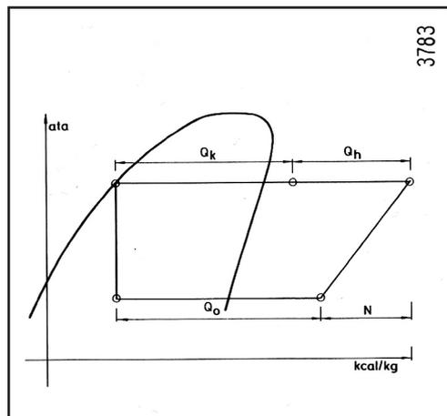
The object of the condenser in the refrigeration system is to remove the heat supplied to the refrigerant in the evaporator and during the compression in the compressor, as well as to condense the refrigerant vapours into liquid.
