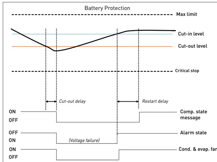
For initial startup after power ON, extra protection has been provided by allowing cut-in only when the voltage exceeds cut-out + 1 V DC.
