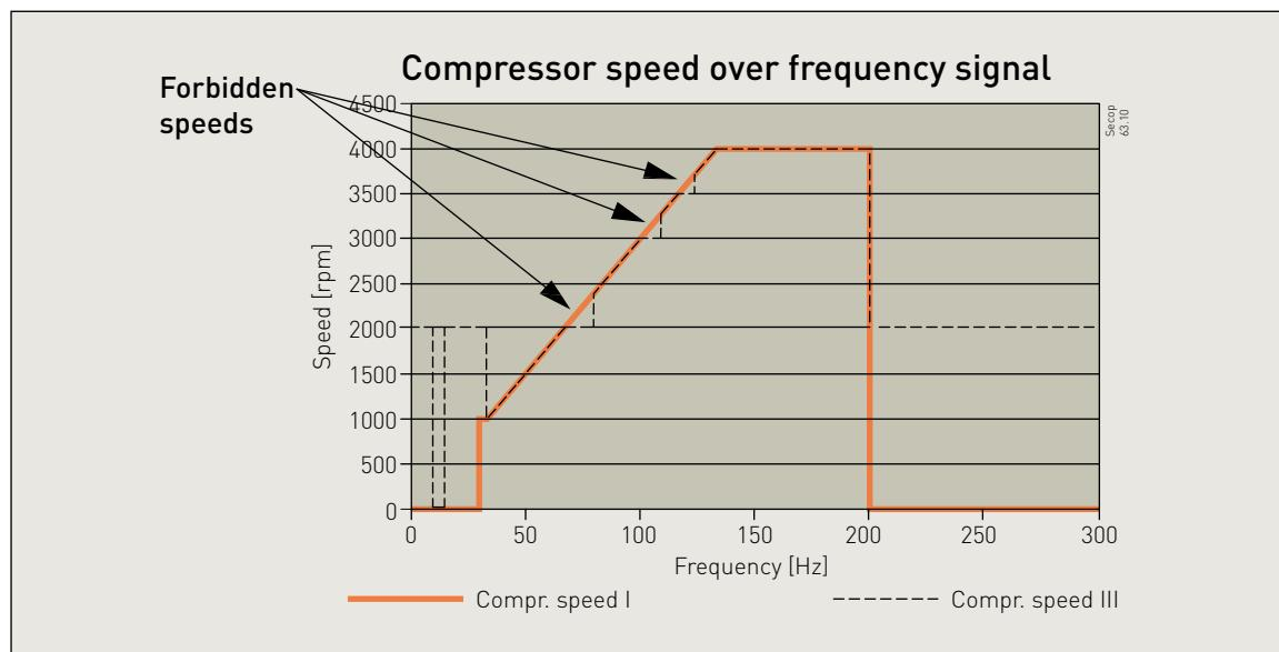
Tip: If a multimeter is connected to the frequency input wires, the display will show what frequency is critical, related to motor speed at which the cabinet causes resonances.
