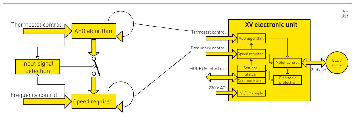
The thermostat is the input interface for the AEO. The thermostat switch can be a mechanical thermostat or a relay (or triac/FET) in an appliance electronic thermostat.
