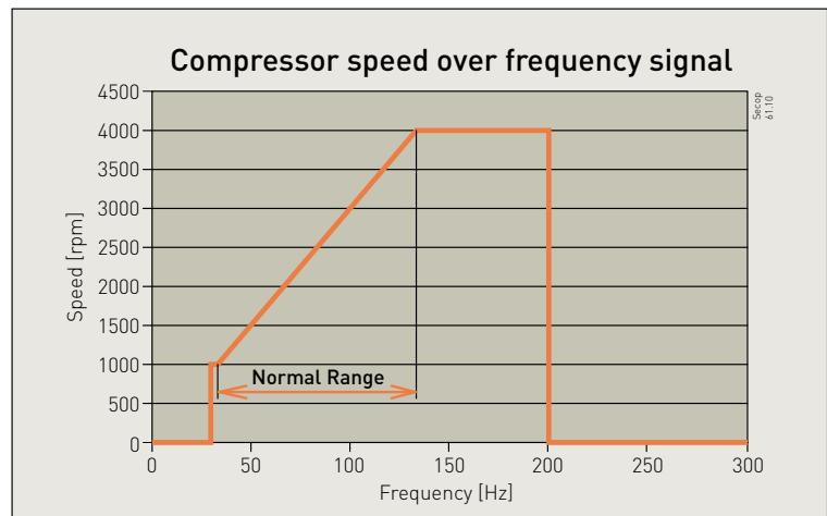
Some speed and cooling capacity settings can be changed via the communication interface (Modbus).
