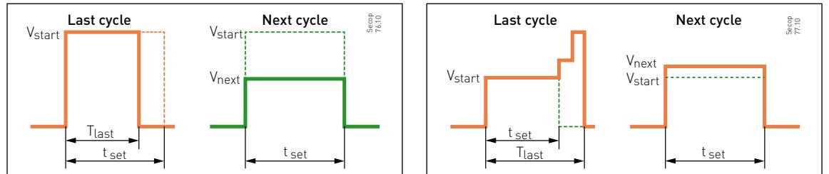
d. The speed boost mode helps to decrease speed rapidly if the last cycle was much too short (an empty cabinet), or it will enable a faster reaction on for example heavy load changes.
