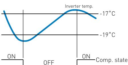
The temperature limits cannot be changed but the actual PCB NTC temperature can be seen and the actual error can be read. See more in the section "PNU number overview – parameters".
