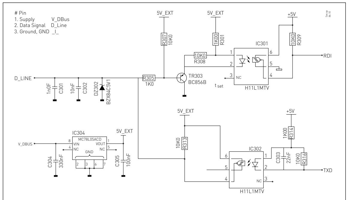
The gateway 105N9501 can be used to connect a PC with Tool4Cool® directly to the XV attached electronic unit. It is a galvanic isolated connection. See separate operation manual to make the Tool4Cool® connection.
