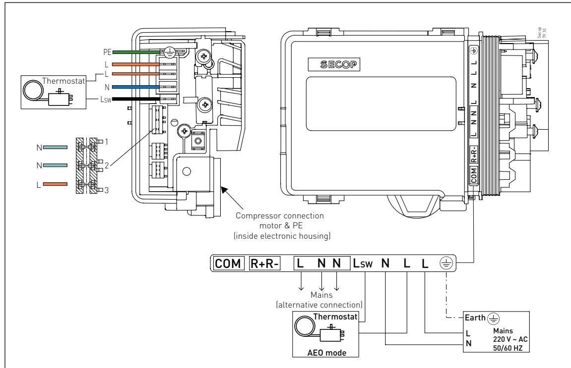
The XV electronic unit is designed to have permanent mains supply. It must not be switched as often as, for example, cut-in and cut-out of a thermostat, due to risk of excessive inrush current and damaged relay contacts. If the appliance electronic is able to connect/disconnect mains to the XV electronic, the duration between switching off and on must be considered.
