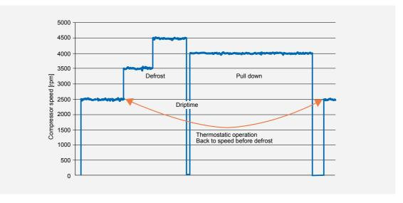
When variable-speed compressors are used in self-adapting capacity modes, defrosting may not work properly since the compressor speed cannot be controlled during defrost: The compressor lacks capacity for hot gas and the following pull-down.
