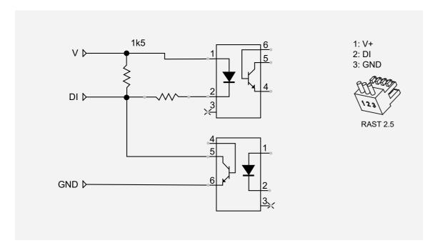
The serial communication is implemented as a single wire half-duplex line—transmitting and receiving on the same line.
