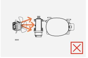
Ensure proper airflow of 3 m/s at both compressor and electronic units.
