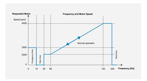
The speed can be controlled by applying a low voltage frequency signal to the frequency input
