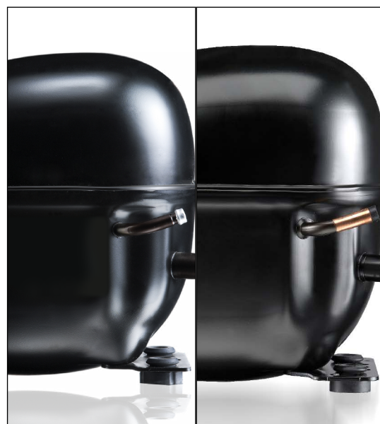
Fig. 2 N-Series compressor with copper-plated steel discharge connector (with aluminum cap) on the left and full copper discharge connector (with rubber plug) on the right
