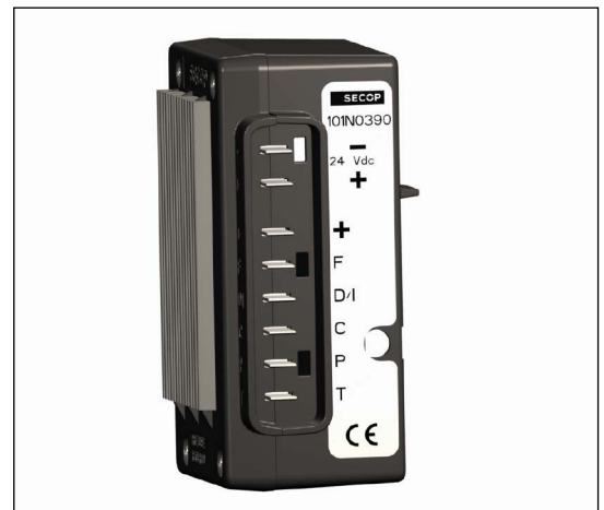
Fig.2 New 101N0390 electronic unit
