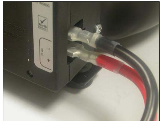
Fig.3 Connectors mounted "back to back"
