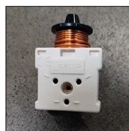
Fig. 3 Existing starting relay, type 117U6xxx/117U7xxx
