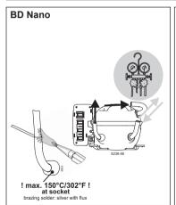
Do not heat up the bottom of the discharge connector directly.
